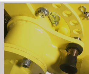
Defoliation head is adjustable from vertical to horizontal
